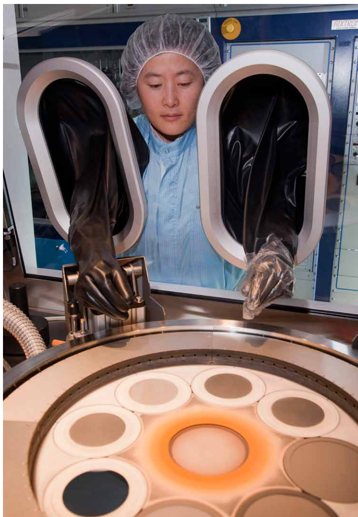
◀ Multi-wafer reactor at FBH for metal organic vapor phase epitaxy of GaN
