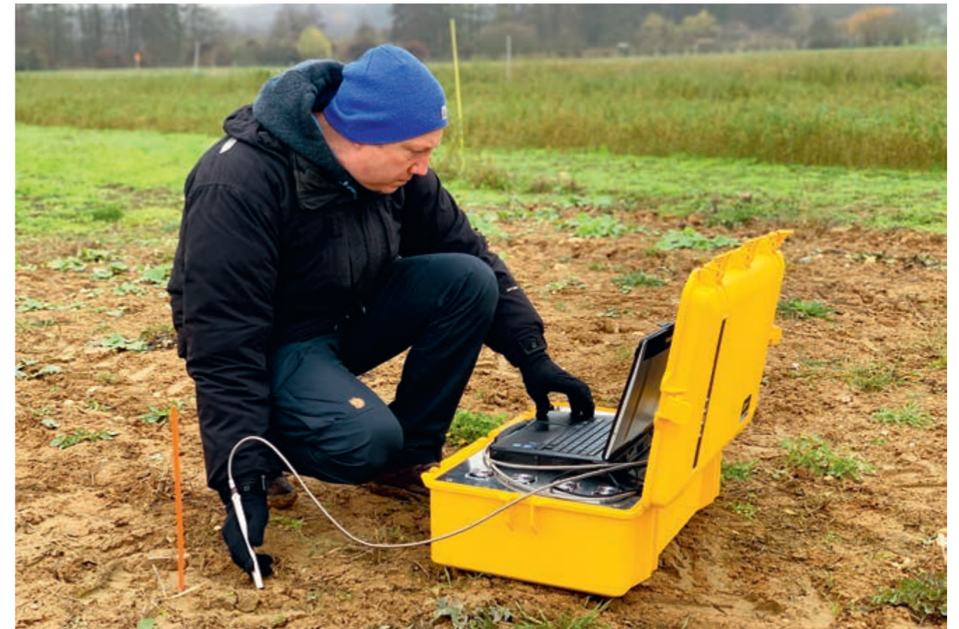
Fig. 1. In-house developed and realized portable SERDS sensor system applied in a real-world test. The system successfully performed on-site SERDS measurements under field conditions.
