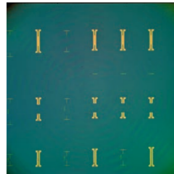
Fig. 2. A set of on-wafer calibration standards: Structures on top and in the middle are reflect standards such as 'open' and 'short', whereas the elements at the bottom are lines with a defined length.
