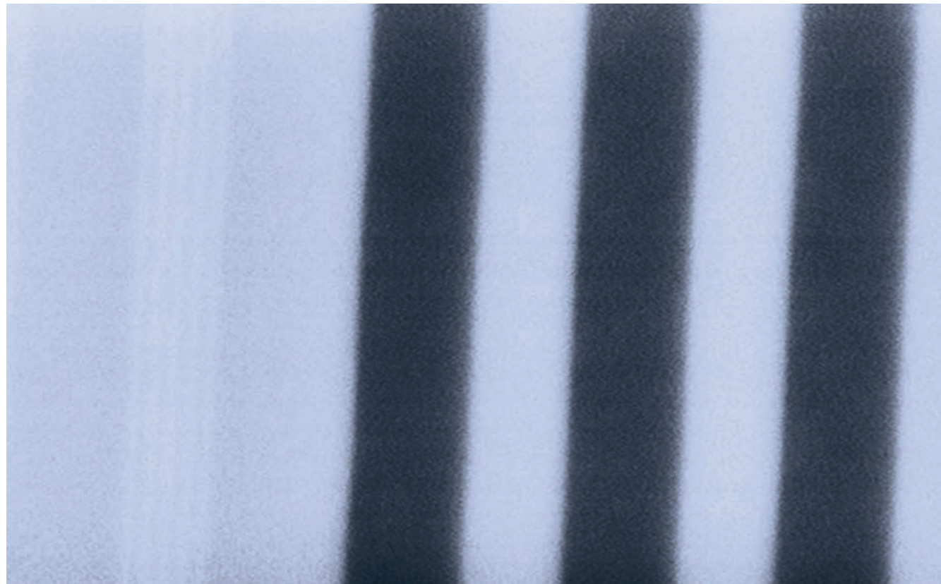
④ Representative secondary electron microscopic cross-sectional image of an (In,Al)GaAs-based SESAM recorded in back-scattered electron mode.
