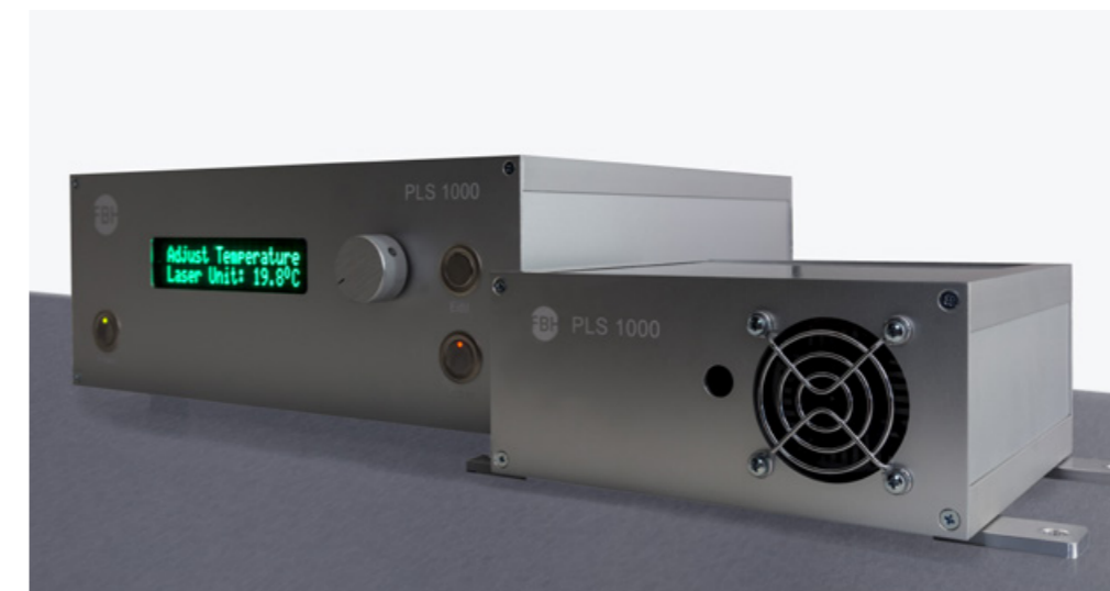
◀ Ready for use – pulse laser system assembled by the Prototype Engineering Group, comprising the main control unit (left) and the optical component (right).
