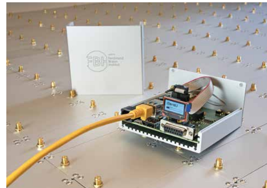
Fig. 2. iSensU (intelligent Sensor Unit) provides connectivity to analog sensors, legacy resources, and digital sensors.
