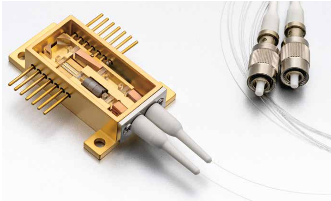
Fig. 1. Fiber-coupled amplifier micromodule with integrated second harmonic generation for super-resolution microscopy.
