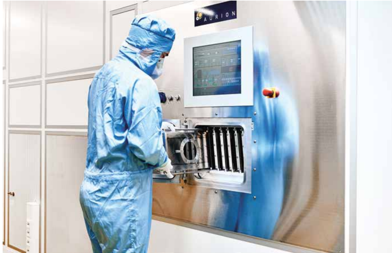
Fig. 1. Loading the sputter tool with 100 mm wafers clamped on carriers.
