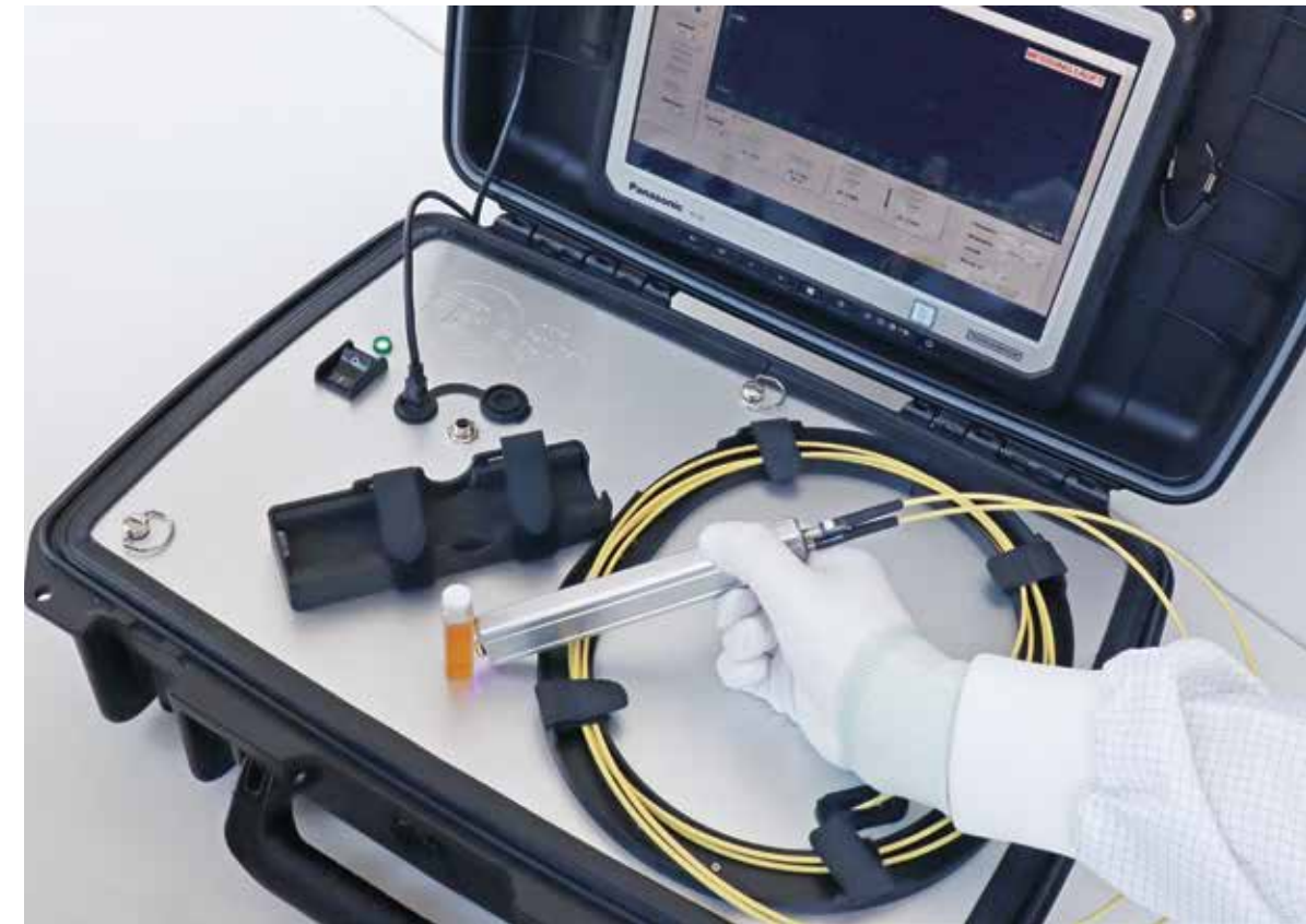
Portable, spectrometer-free resonance Raman system for on-site measurements on selected substances.
