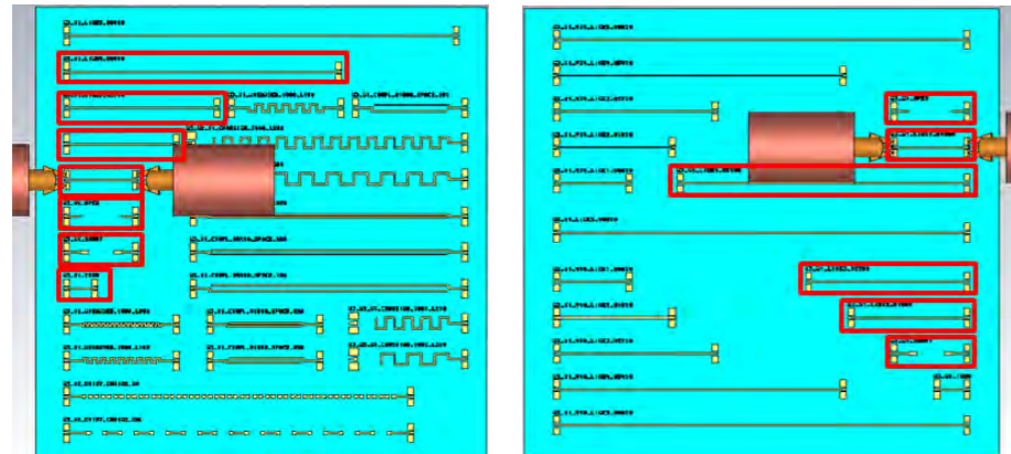
Fig. 1. Same calibration set arranged in two different configurations (left: Cal 1, right: Cal 2).
