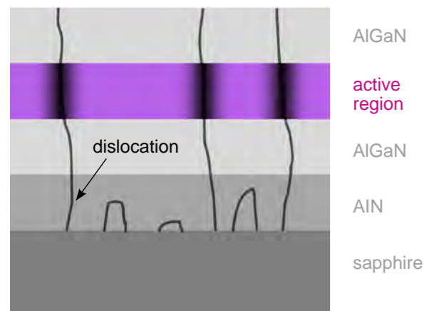
Fig. 1. Simplified schematic, cross section sketch of an LED structure. Threading dislocations propagate from the AlN/sapphire interface into the active region and hinder light generation (dark areas).
