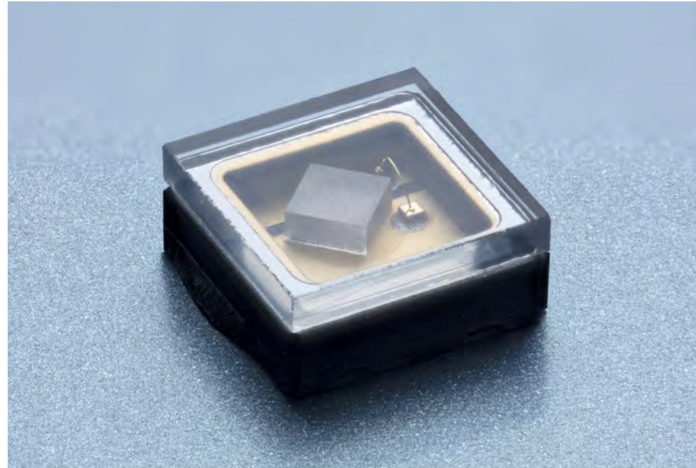
Fig. 1. AlN SMD cavity package with soldered 1 \times 1 \text{ mm}^2 UVB LED chip, Zener diodes for ESD protection and glass lid.
