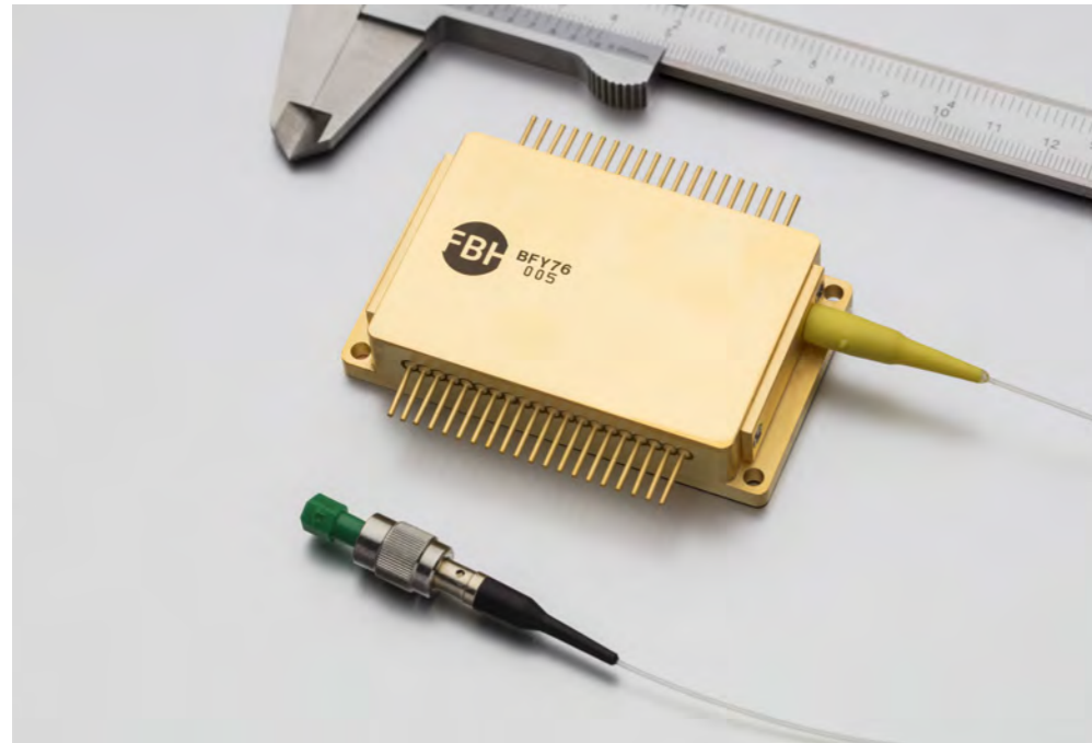
Fig. 1. Diode laser module emitting at 561 nm in a butterfly package.
