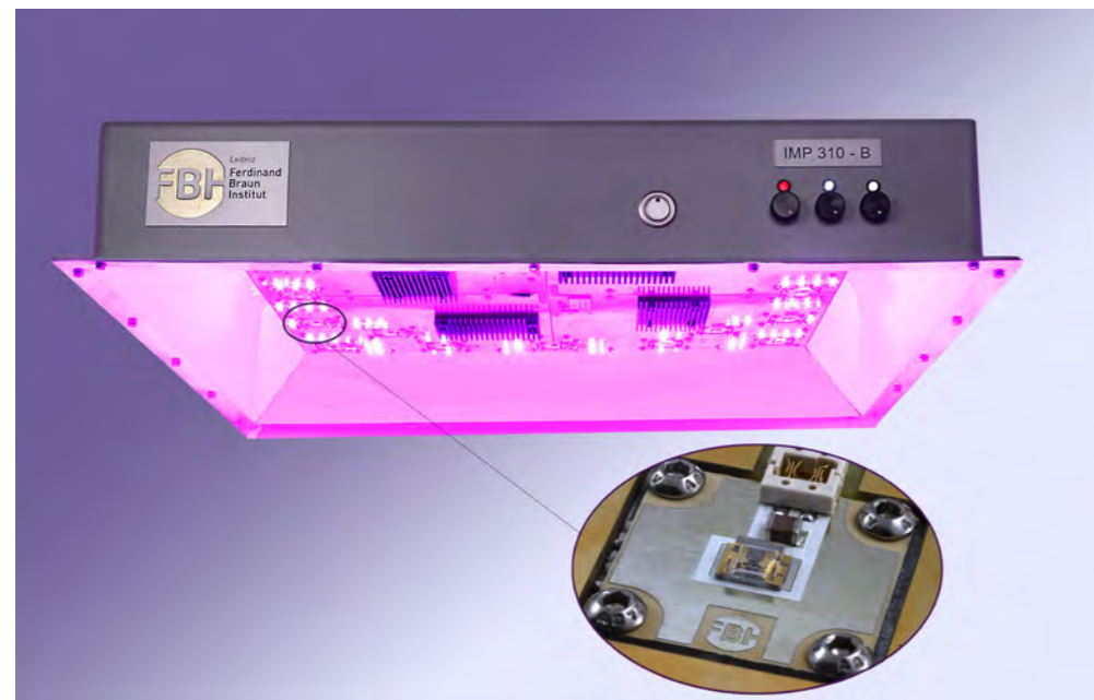
LED module for plant growth lighting providing light of different wavelengths: UVB (310 nm), blue (451 nm), red (660 nm). LED-Modul zur Pflanzenbestrahlung mit Licht verschiedener Wellenlängen: UV-B (310 nm), blau (451 nm), rot (660 nm).
