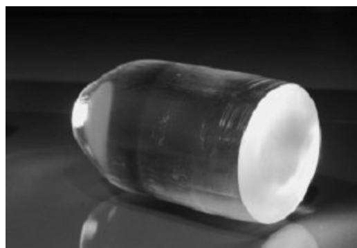
Fig. 1 2 inch \text{LiAlO}_2 crystal of 80 mm length.
