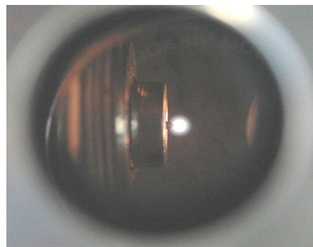
Fig. 5. Upper part of the resonator with a plasma flame on top of its inner conductor.
