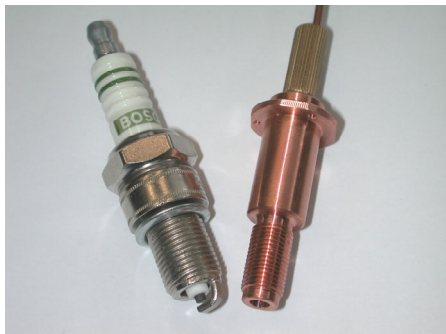
Fig. 4. Packaged resonator in comparison with a conventional spark-plug.
