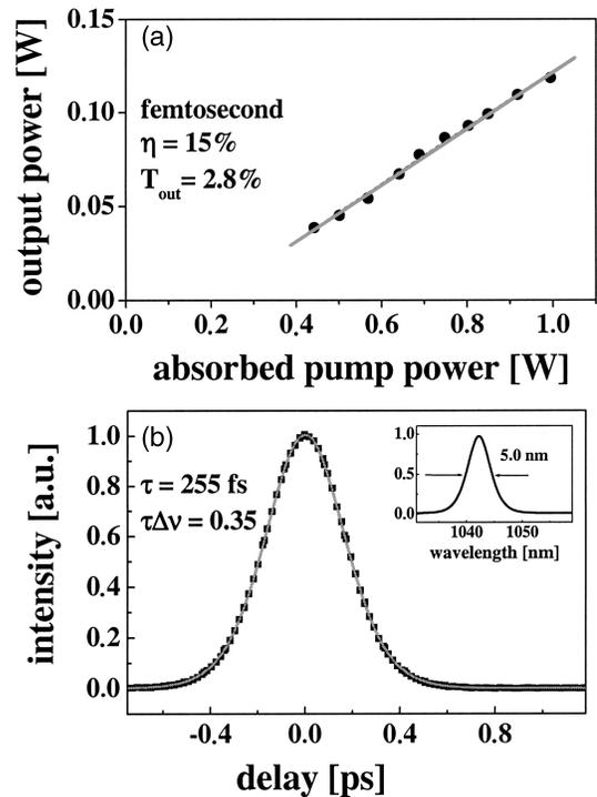
Fig. 4. Performance of the Yb:Sc<sub>2</sub>O<sub>3</sub> mode-locked laser with the TDL as the pump source in the femtosecond regime. (a) Output power versus absorbed pump power. (b) Autocorrelation trace and spectrum (inset).
