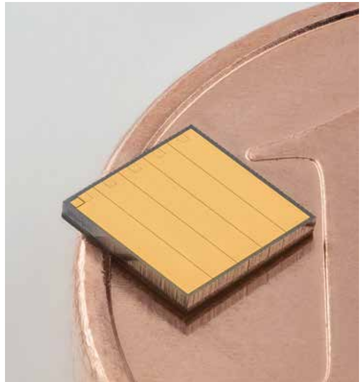
Vertical GaN high current power switching transistor for direct laser pulsing
