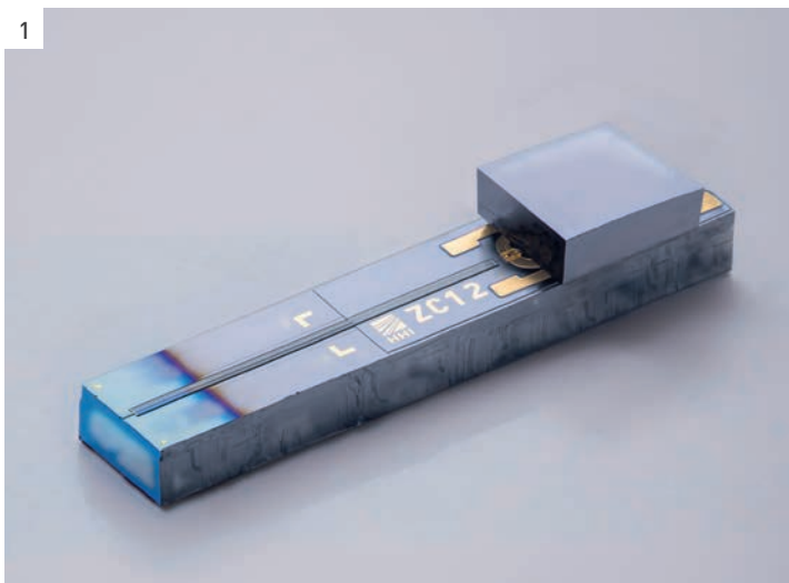
Heterointegrated InP-based transimpedance amplifier (TIA) on a photo diode receiver using FBH's heterointegration process. The complete system offers broadband operation from DC up to 80 GHz.
