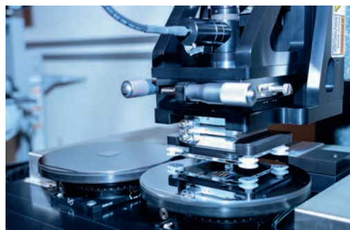
X-Celeprint micro-transfer printer in use at FBH.
