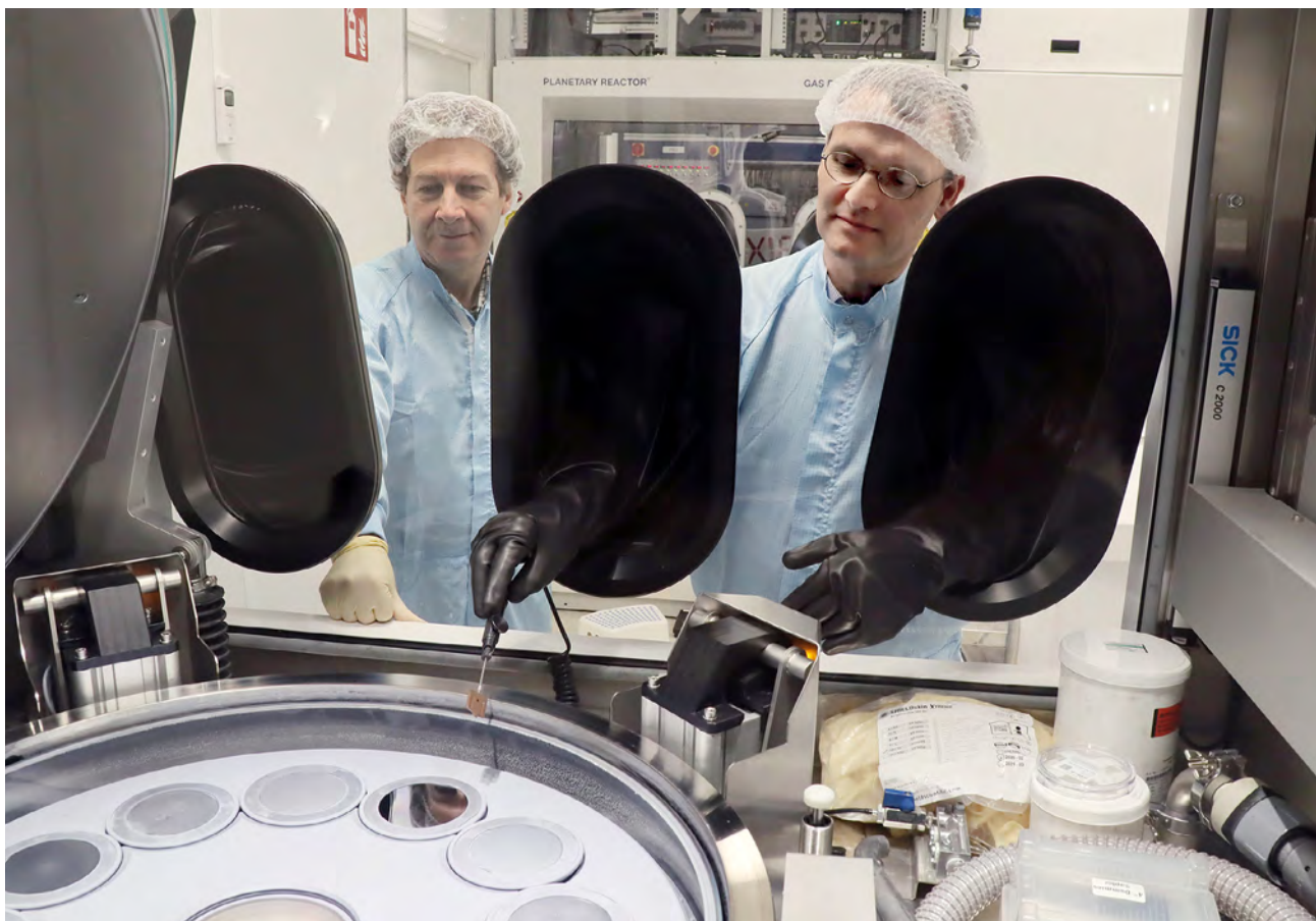
In our epitaxy lab, we grow ultrathin semiconductor layers with precisely defined crystalline properties.
