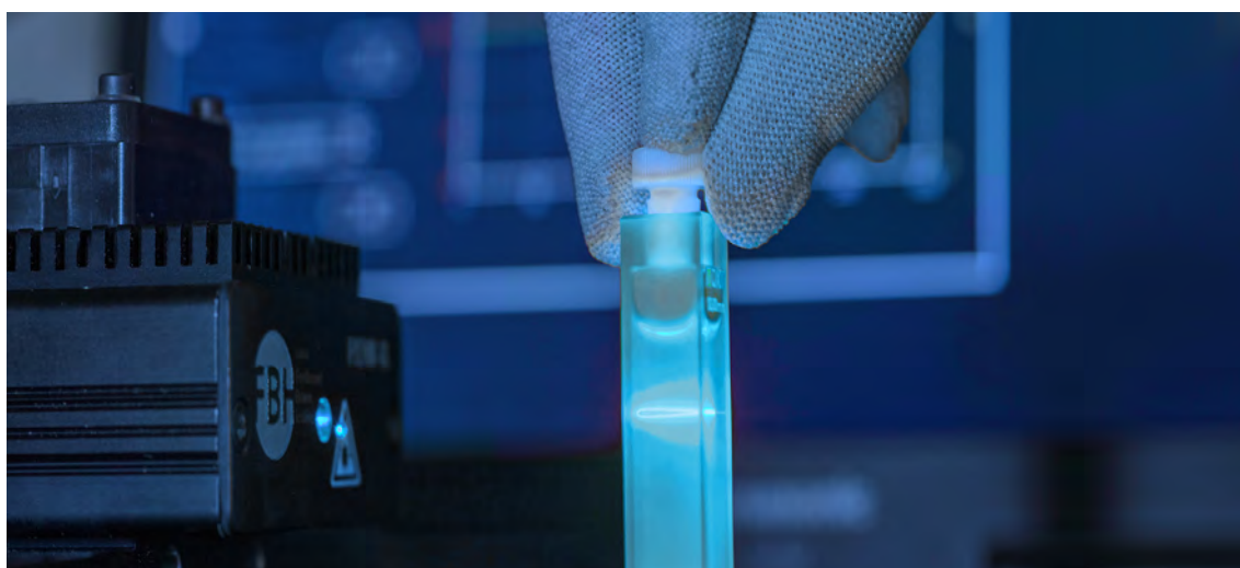
Diode laser turn-key system with integrated dual-wavelength laser used for Raman spectroscopy and SERDS investigations.
