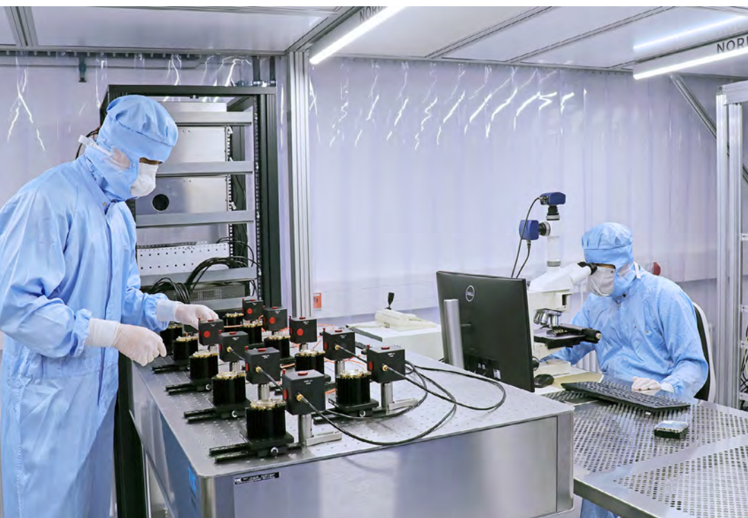
ISO 5 cleanroom laboratory for reliability testing of diode lasers for space missions.
