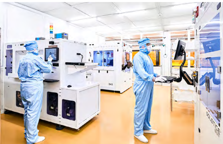
Automated tools for wet chemical and electroplating processes to ensure superior reproducibility.
