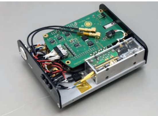
Fully autonomous, frequency-stabilized laser source for quantum sensors and atomic clocks.
