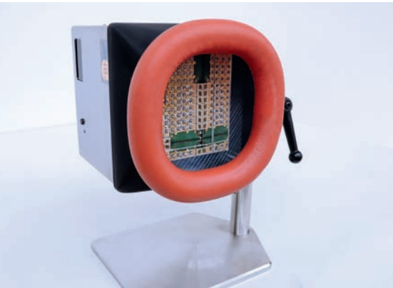
Far-UVC LED irradiation system for medical tests on human skin.
