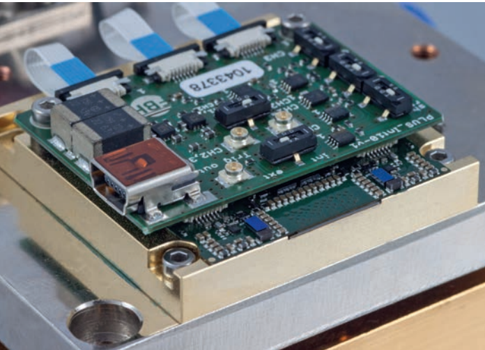
Laser module with integrated driver for automotive LiDAR applications.
