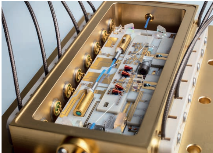
Remarkably robust – micro-integrated, frequency-stabilized diode laser module used for precision experiments in space.
