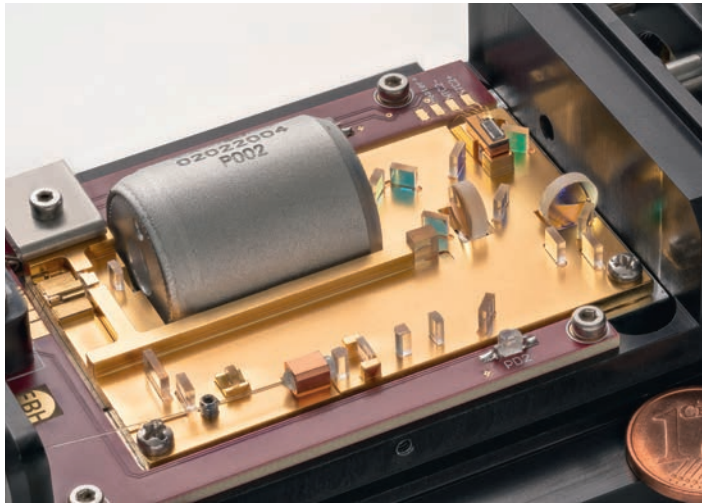
Quantum light module for generating entangled photons, with built-in laser source and quantum interferometer.
