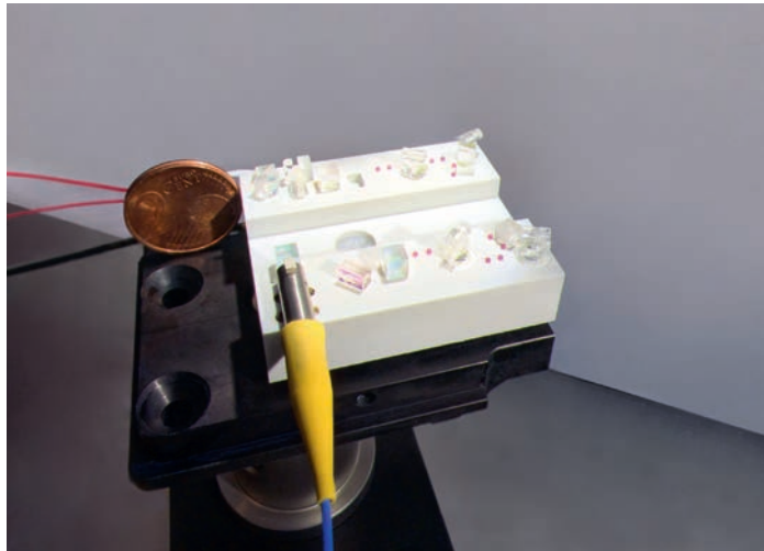
Compact, micro-integrated crossed beam optical dipole trap with a volume of less than 25 ml.
