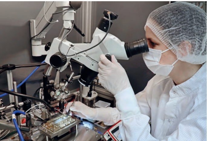
High-precision micro-assembly of photonic modules for space applications.
