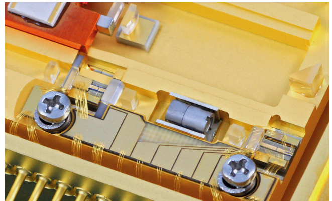
➤ Master oscillator power amplifier module with SHG crystal
