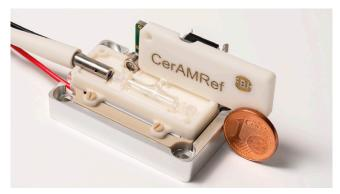
Micro-integrated CerAMRef spectroscopy module. The micro-optical bench and enclosure lid are 3D-printed from Al<sub>2</sub>O<sub>3</sub> ceramics.
