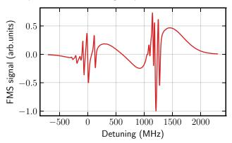
Doppler-free frequency modulation spectrum of the Rb D2 line, obtained with the CerAMRef reference module and plotted over the frequency detuning. This spectrum exhibits features from the <sup>87</sup>Rb D2 F = 2 → F' and <sup>85</sup>Rb D2 F = 3 → F' transitions.
