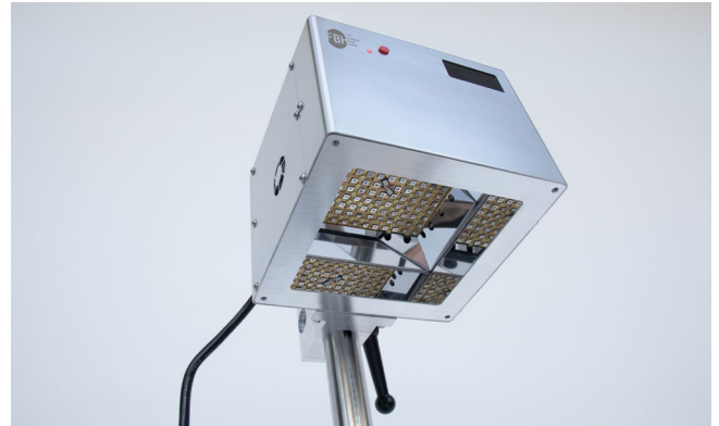
➤ Prototype of the far-UVC LED irradiation system to fight multidrug resistant pathogens.
