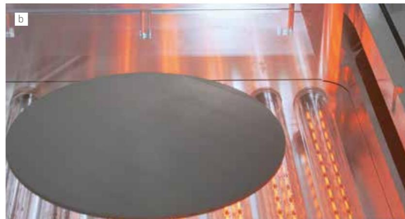
Fig. 4. (a) Wafer chamber of the high-voltage implantater. (b) Graphite box containing a wafer in the RTA chamber. The glowing halogen lamps are used to rapidly heat the wafers to high temperatures.
