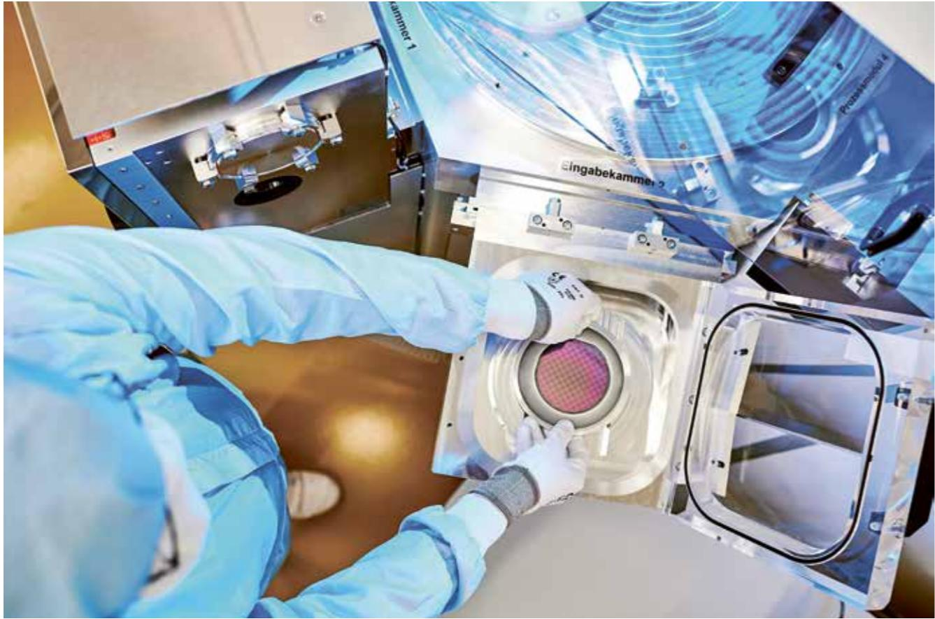
⌚ Cluster tool for atomic layer deposition of extremely thin films in FBH's cleanroom-2.
