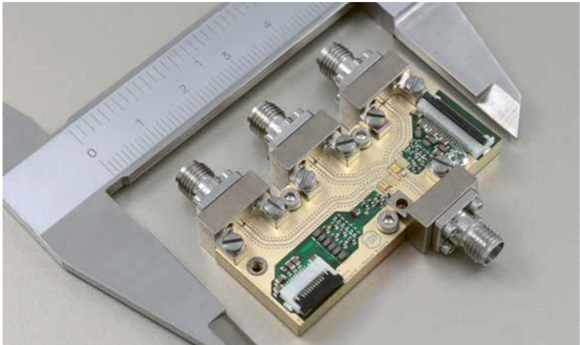
Compact digital GaN-based class-E outphasing PA module; size: 50 x 45 mm<sup>2</sup>.
