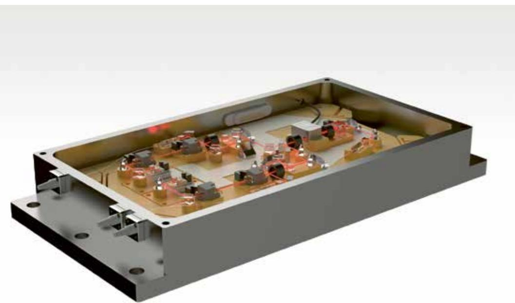
Fig. 1. CAD model of the SOLIS-1G repumping module. Dimensions are ca.  $200 \times 100 \times 30 \text{ mm}^3$ .
