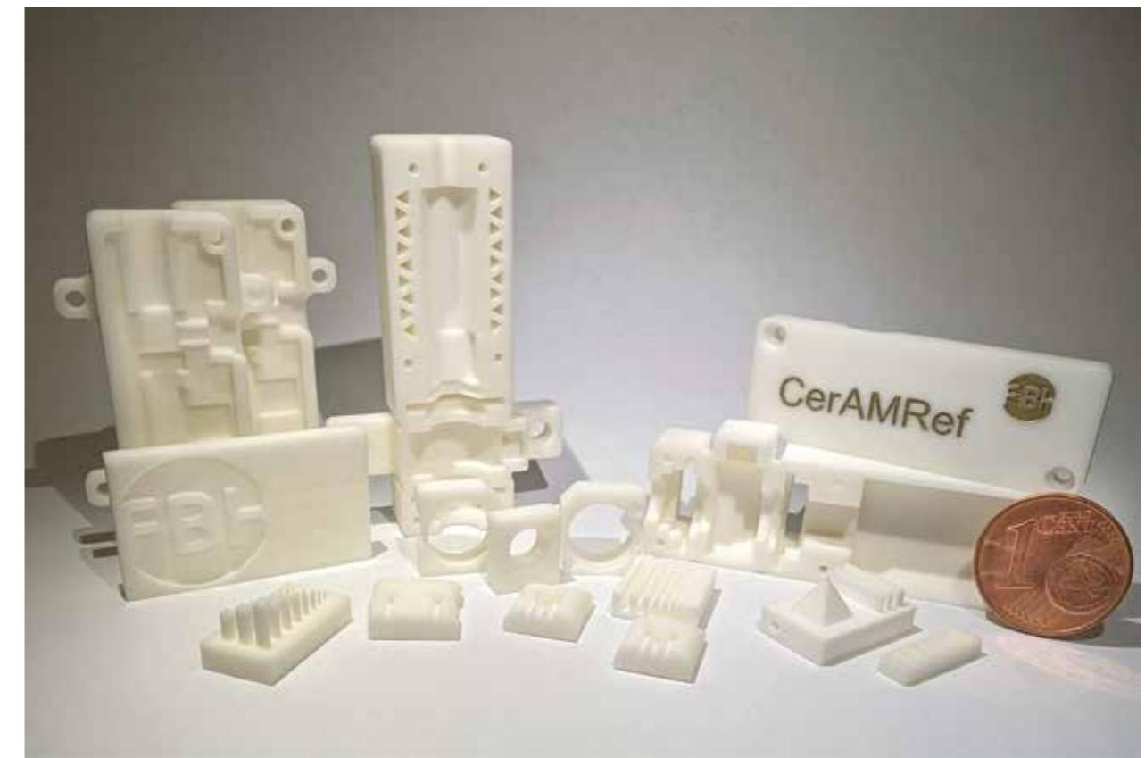
Fig. 2. Additively manufactured alumina ( $\text{Al}_2\text{O}_3$ ) example components, including micro-optical benches, mounts for electro-optical components, and test structures to optimize print and post-processing parameters.
