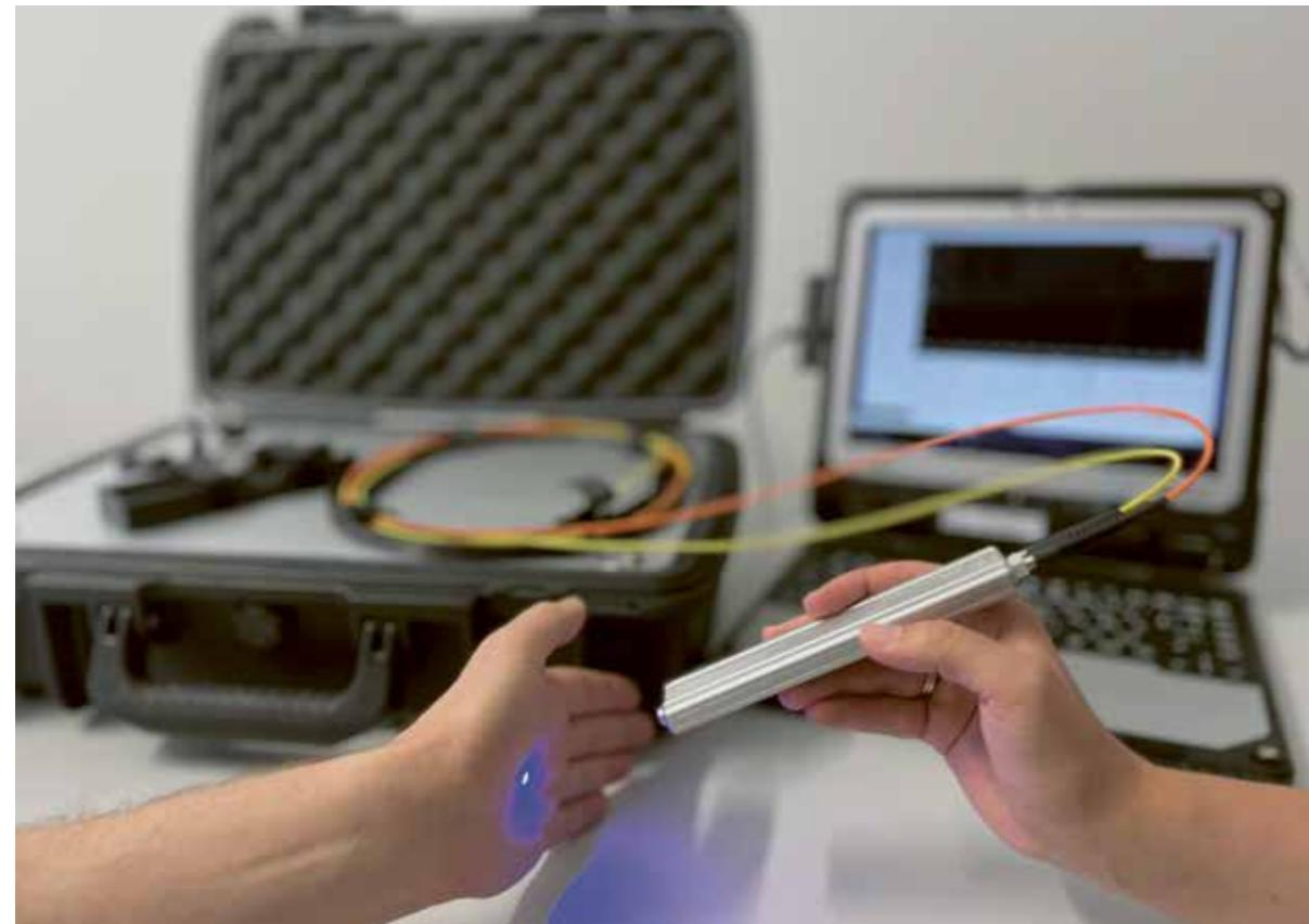
Determines the concentration of carotenoids in the skin: real-life test of FBH's mobile, spectrometer-free resonance Raman system.
