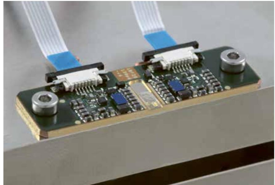
Fig. 1. FBH's nanosecond pulsed laser driver integrated with a soldered and bonded 1 mm long DFB BA laser for LiDAR applications.
