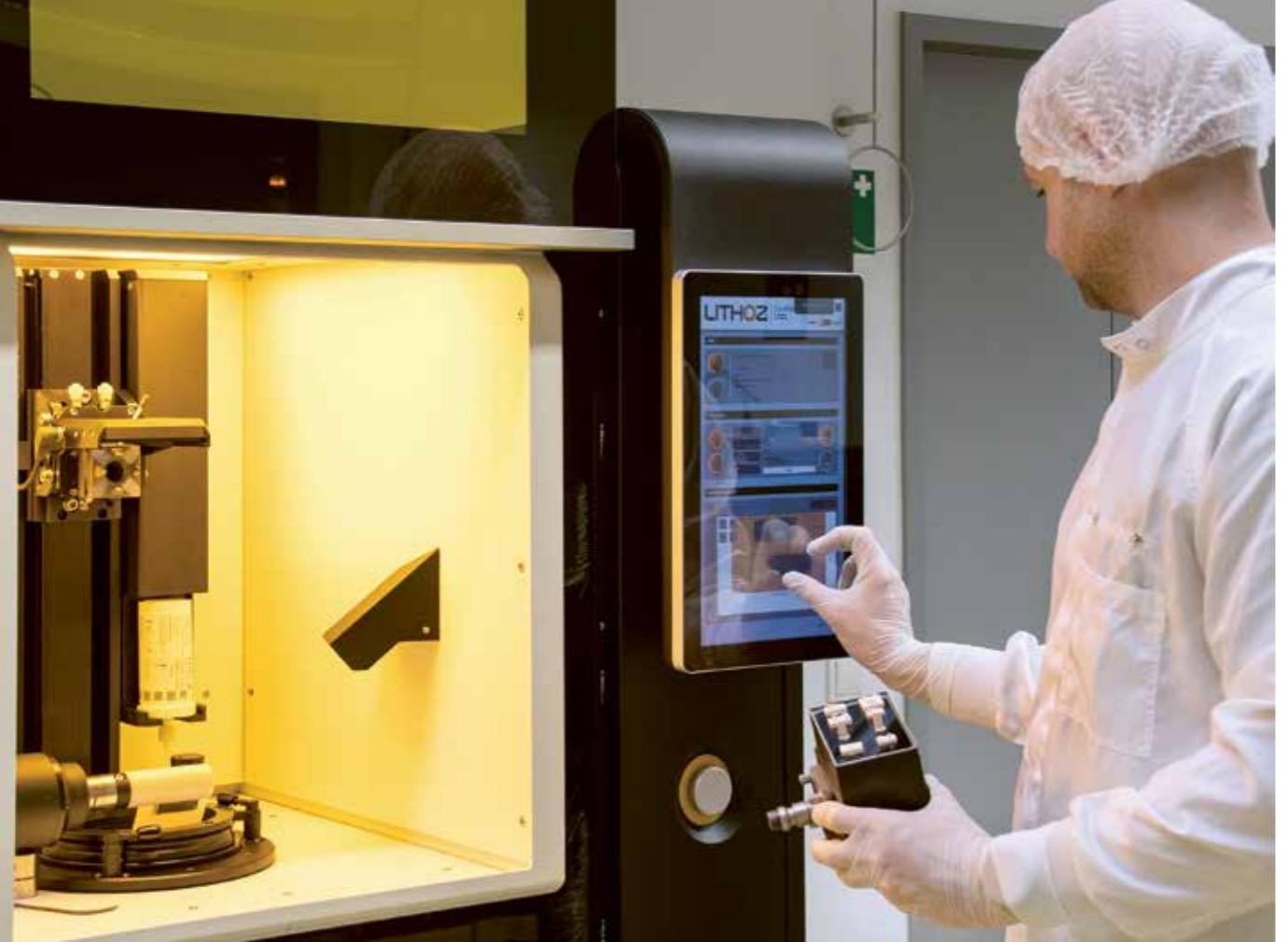
High-precision ceramic 3D printing at FBH: We used this lithography-based printer to realize the micro-optical bench of the miniaturized optical frequency reference.
