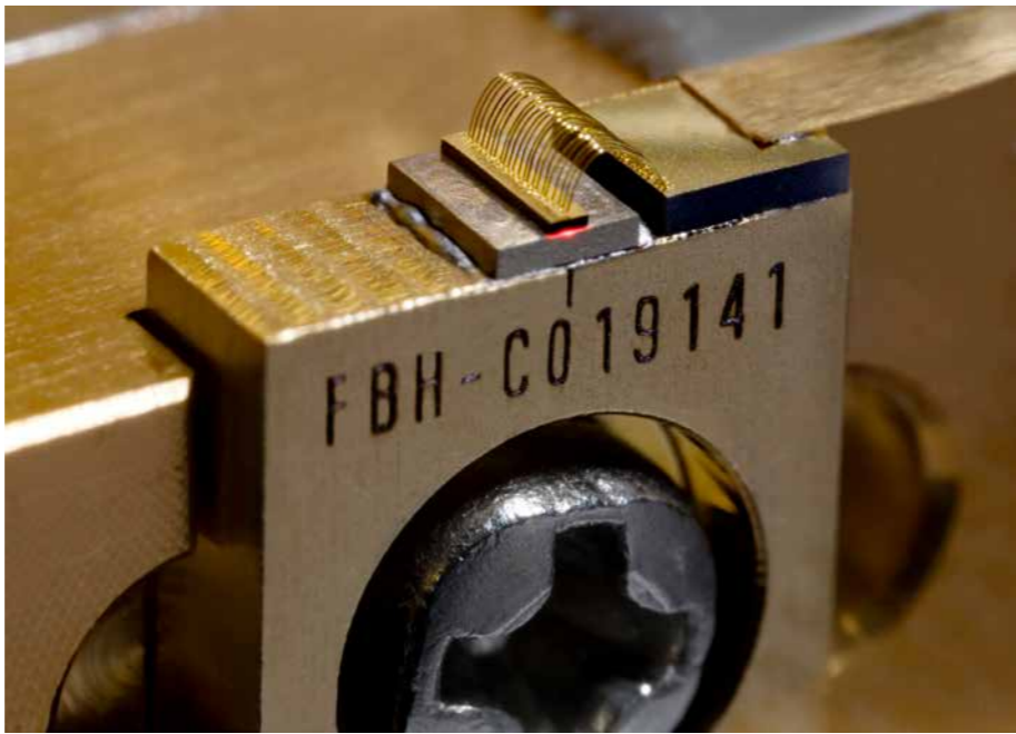
Fig.2a) Diode laser with orange emission typical for this wavelength.
