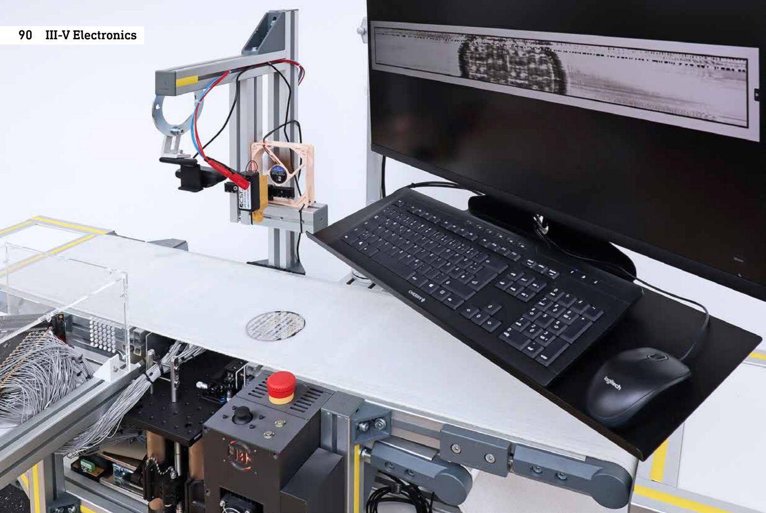
Fig.1. The terahertz line scanner captures a structured wafer in real time.
