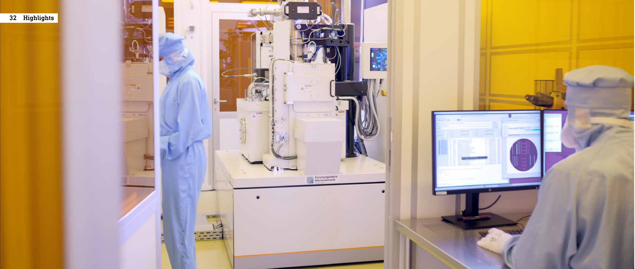
E-beam lithography system in FBH's cleanroom to create innovative device concepts – enables structuring down to the sub- \mu\text{m} range.
