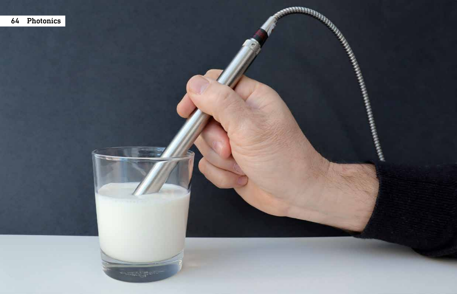
Fig. 1. Raman probe of the portable SERDS sensor system directly immersed into a milk sample.
