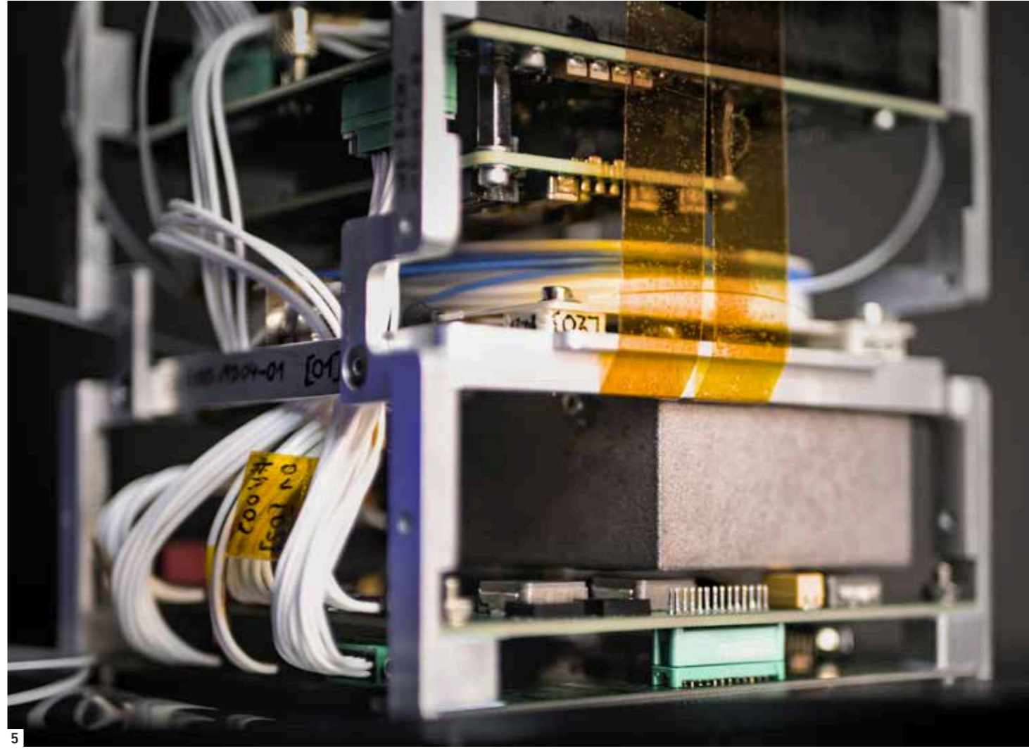
Fully assembled, very compact Quick 3 payload with dimensions of only 10 x 10 x 15 cm 3 , including single-photon source and quantum experiment. The gray box contains the FBH laser unit.
