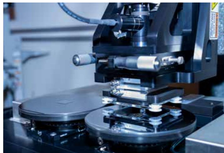
Fig. 3. Photograph of our X-Celeprint micro-transfer-printing tool in the process of transferring laser chiplets from a GaAs source wafer to a six-inch target wafer.
