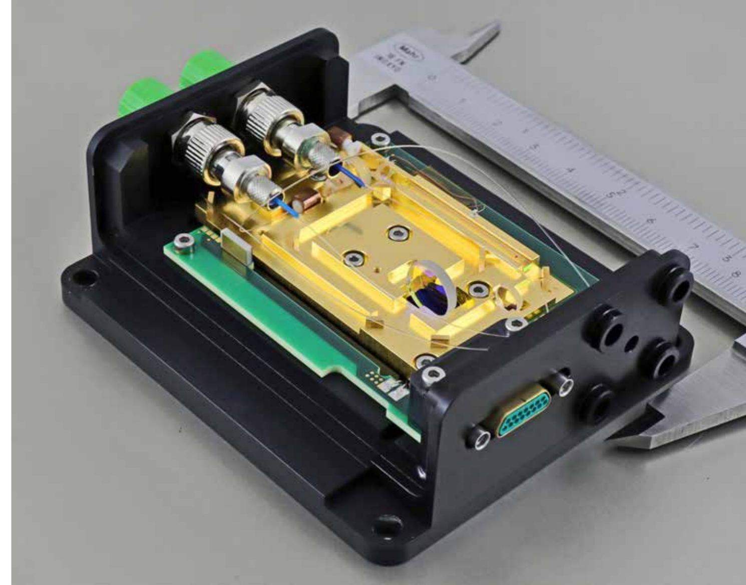
Fig. 1. Quantum light module with nonlinear crystal, folded reference path and fiber connectors integrated into the housing for simple delivery of pump radiation and quick connection to the spectrometer.
