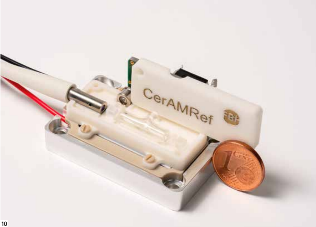
Miniaturized optical frequency reference module with rubidium vapor cell, enabled by additively manufactured technical ceramics.
