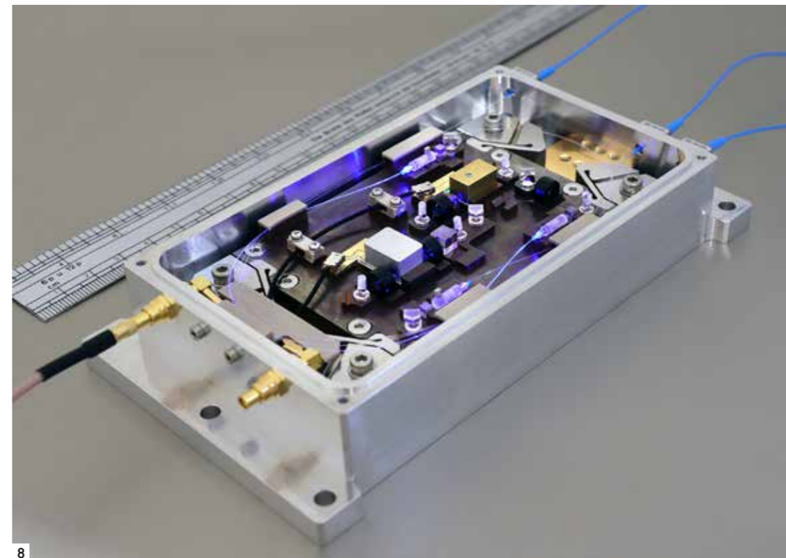
8 461 nm light-control unit for strontium-based optical clocks, targeting space applications.
