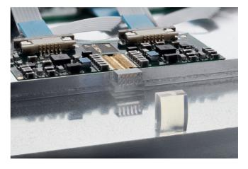
FBH high current ns laser driver with integrated ridge-waveguide laser diode – output power of three emitters is collimated into one spot by optical components from FISBA Photonics GmbH
