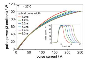
Optical pulse power vs. driver pulse current width from a three emitter bar for different pulse lengths. Inset: optical pulse power in dependence on current pulse width
