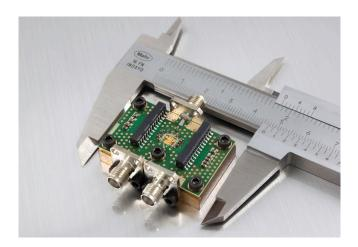
Highest linearity reached: digital transmitter module including digital PA chip, output bandpass filter and T/R switch.
