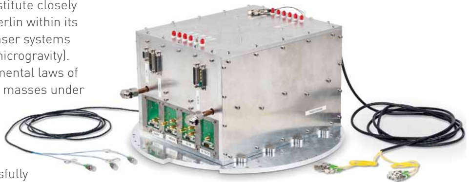
MAIUS laser system developed by HU Berlin with integrated DFB-MOPA laser modules from the FBH used to successfully create a Bose-Einstein condensate for the first time in space
