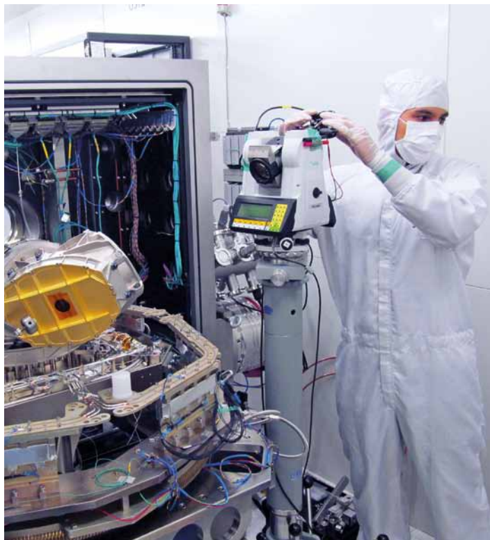
Laser communication terminal (LCT) integration and testing in Tesat-Spacecom's cleanroom
