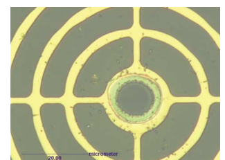
Sapphire target hit by a single laser shot (front-to-backside alignment). The deviation center-to-center is X-0.4 \mu\text{m} and Y+0.4 \mu\text{m} .
