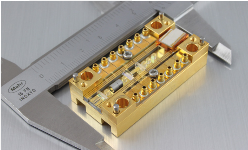
• Diode laser module emitting in the yellow spectral range, e.g., for treatment of eye diseases by laser coagulation.
