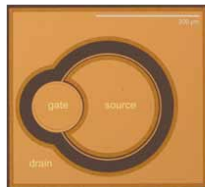
SEM viewgraph of a circular MISFET fabricated on n-doped gallium oxide.
