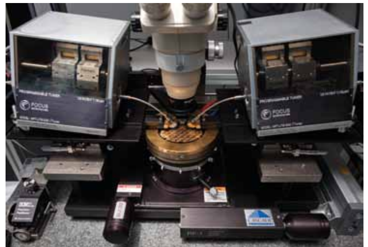
20W load-pull system for device characterization up to 34 GHz.
