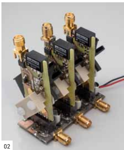
Fig. 2. Modular high-power modulator for multi-level class-G operation. Fig. 3. Class-G discrete envelope tracking system.
