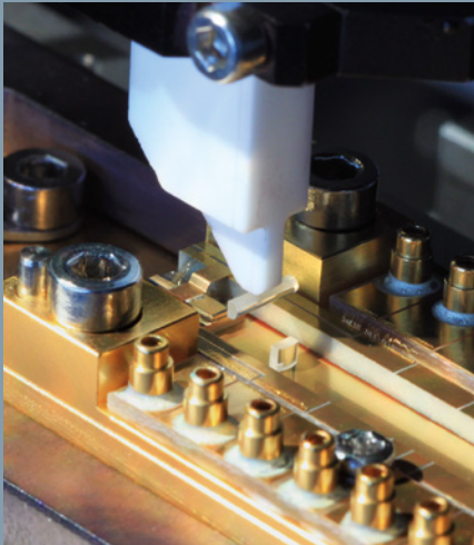
◀ High-precision mounting of a micro lens into a compact diode laser module.
