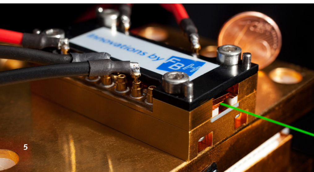
◀ Hybrid-integrated diode laser module for display applications.
