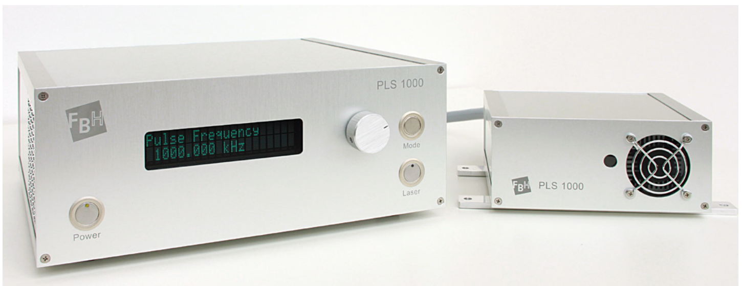
▲ FBH pulse laser system comprising the main control unit (left) and the optical component (right).
