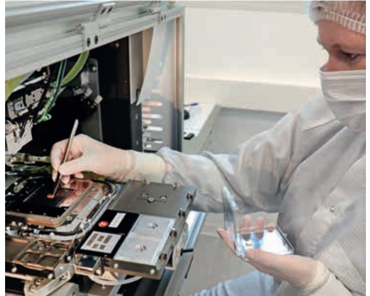
Automated assembly of diode lasers for use in high-power laser stacks.
