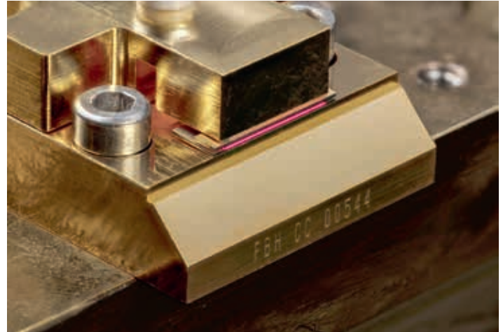
Red laser bars with world-record QCW output power of over 350 W at 665 nm.
