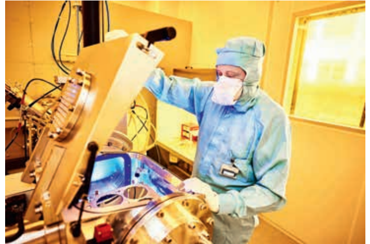
FBH's state-of-the-art implanter, for sophisticated lateral current control.
