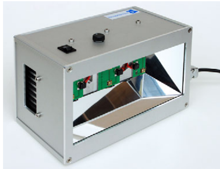
▲ Fig. 1. Prototype of a custom UV-A LED module.
