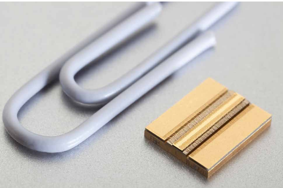
Fig. 1. A new generation of FBH diode laser designs offers very high conversion efficiency at high optical output power. These long cavity lasers are mounted on sub-mounts for use in industrial laser systems.
