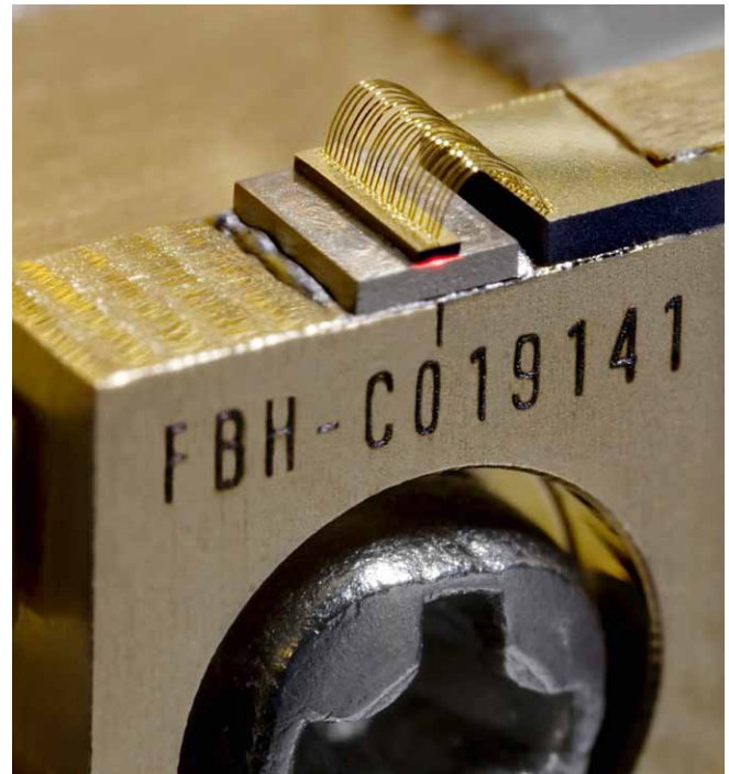
High-power tapered diode laser at 660 nm mounted p-down on CVD-diamond heat spreader and c-mount.
