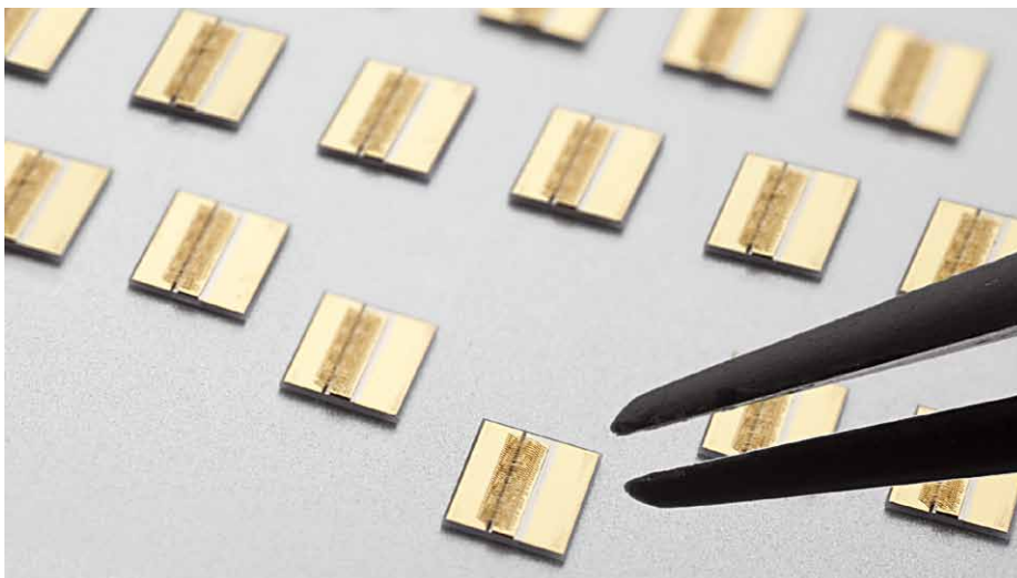
Fig. 1. Diode lasers as pump sources for ultra-short pulse lasers.
