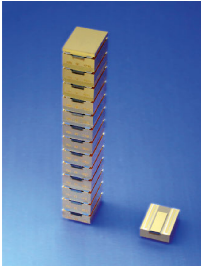
Fig. 1. Exactly aligned laser chip (p-down) and two spacers soldered in parallel on the lower CuW heatsink of a stack element (right). Diode laser stack built on 13 stack elements (left).
