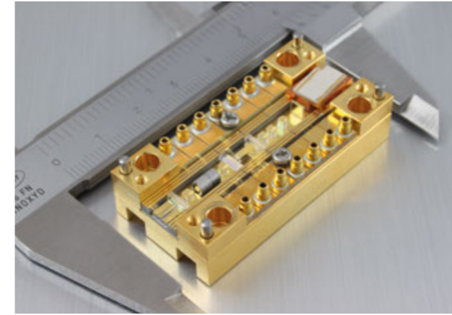
Fig. 3. Module comprising a master-oscillator power-amplifier setup and a nonlinear planar crystal for pulsed operation at 561 nm.
