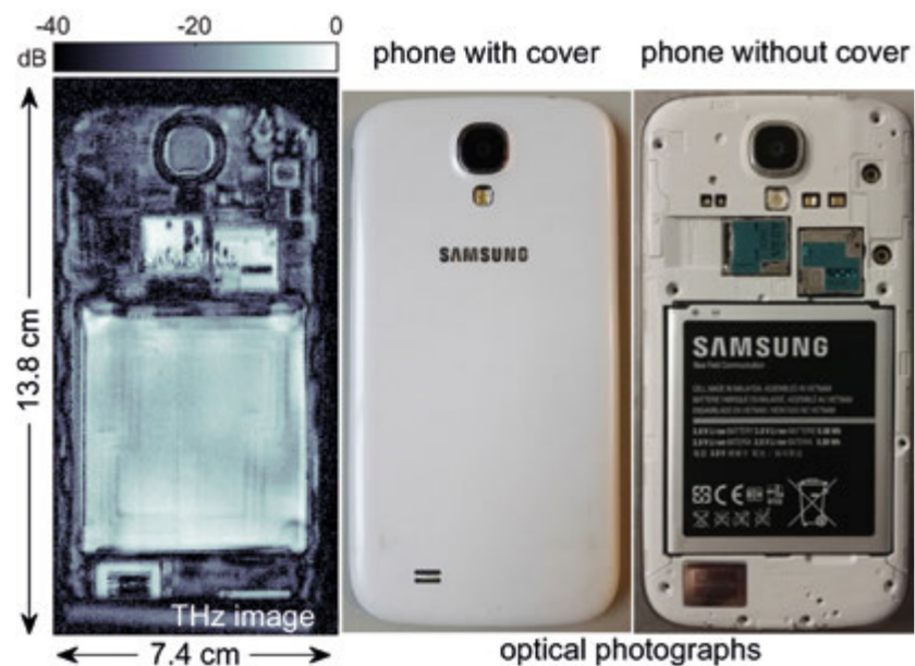
Fig. 2. THz reflection image through cover of a cell phone at 504 GHz.
