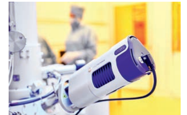
Wafer stepper & scanning electron microscope (SEM) when inserting a mask (top) and detector at the SEM to determine chemical elements (below)
